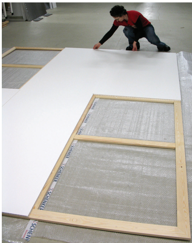
Fig. 5. Constructing mount of paper honeycomb panels glued to a wooden lattice.
