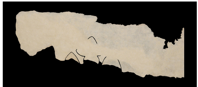
Fig. 17. Image of the fabricated overlay. The paper was cast to avoid covering inscriptions and cut to precision where lines of ink should be exposed.
