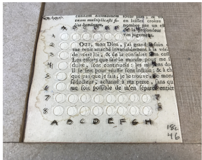
Fig. 4. Polyester film overlay with alphanumeric grid used to avoid the printer’s ink when taking color measurements of the antique gelatin paper samples.
